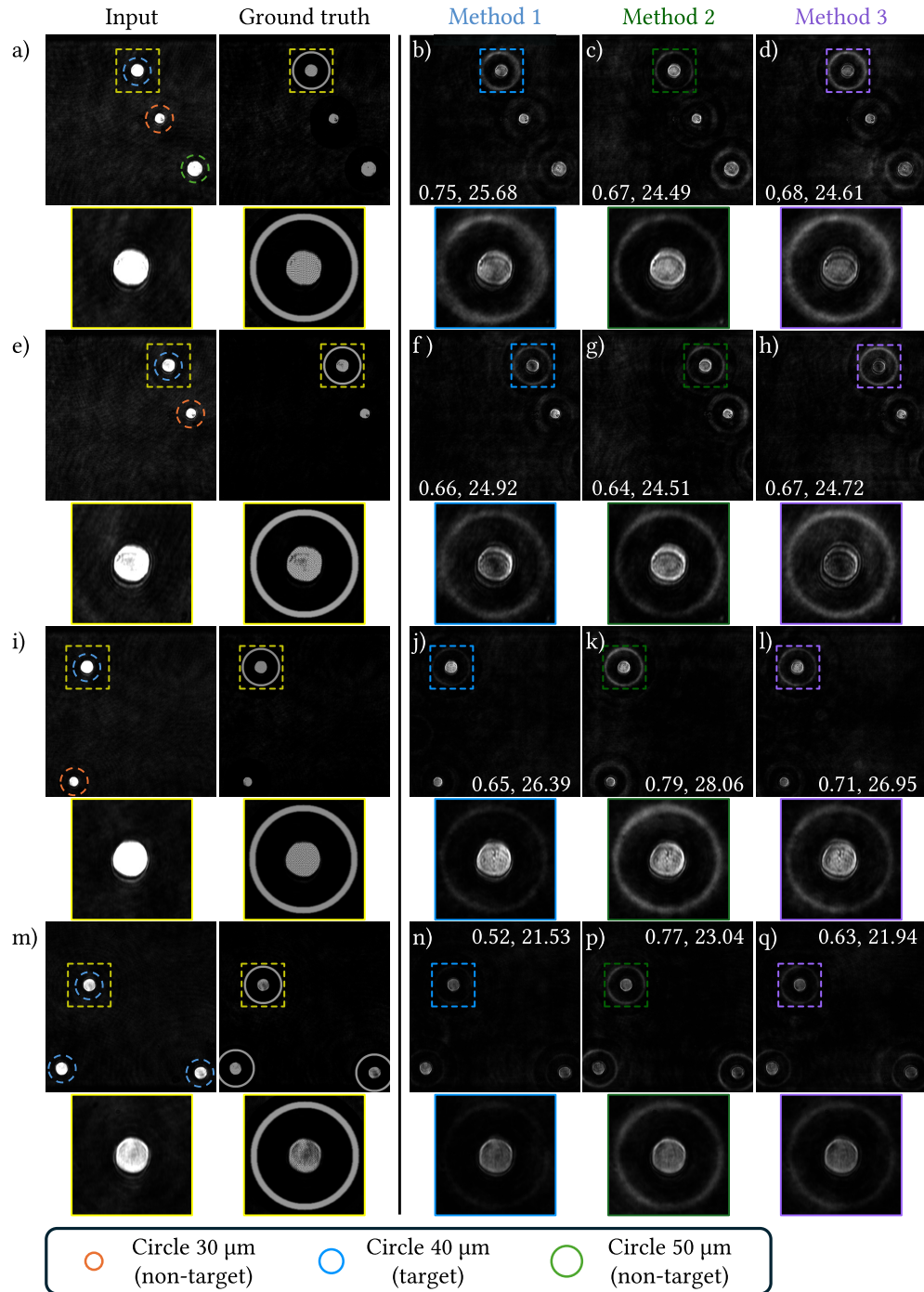
Fig. 5. Scenario 2: Size-based selective object highlighting. We present the evaluation results for each optimization method, captured at an exposure time of 200 ms. Each method employs a phase mask to highlight 40 \mu\text{m} diameter circles. The optimized phase is fixed and applied to different novel scenes. We report CC and PSNR values for each method. See Visualization 1 for a live demonstration of augmentation.
