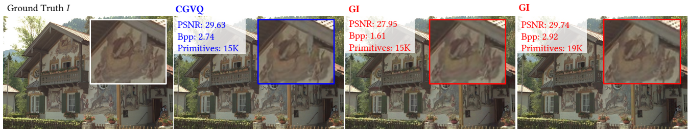
Figure 4: Qualitative Comparison of Reconstruction Fidelity. From left to right: (1) Ground Truth I ; (2) CGVQ reconstruction with 15K primitives; (3) GI baseline with 15K primitives; (4) GI baseline with 19K primitives. Source image © Kodak.
